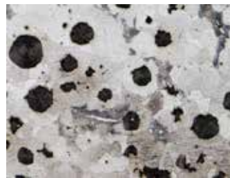
Figure 2 : Malleable Cast Iron, original image before grey scale thresholding.
